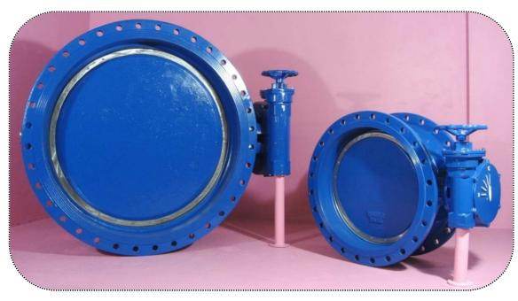
It is a type of valve consisting of a disc travelling 90 degrees on shaft inside of a circular body. It is a type which needs less installation space and which is light in weight and cheap in cost compared to other types of valves.
