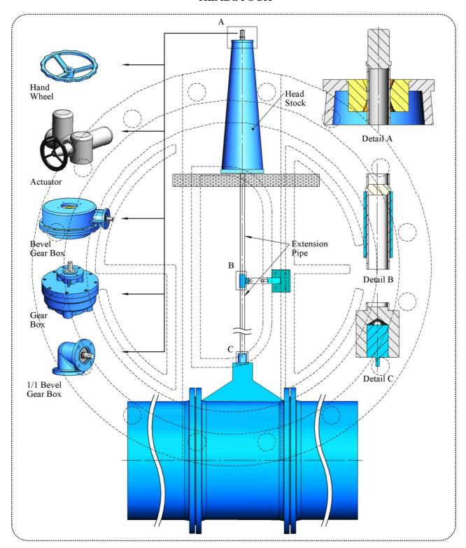
Headstock consists of a cast body, extension spindles and guide brackets holding the spindles.
